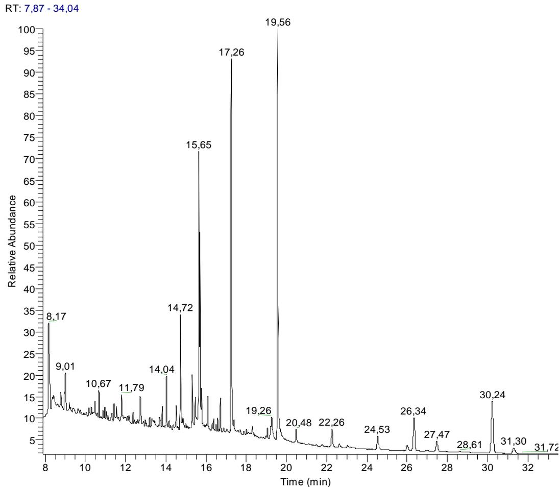
Figure D. An example of a chromatogram, in this case from a sample of dehydrated *R. coronifer*. Both the standard sorbitol and trehalose are detected in this sample. The peak at retention time 15.65 corresponds to the sorbitol standard, while the peaks at 17.26 and 19.56 originate from carboxylic acids, and the trehalose peak is shown at retention time 30.24. The carboxylic acids probably originate from cell membranes (Kjellman 2004).
