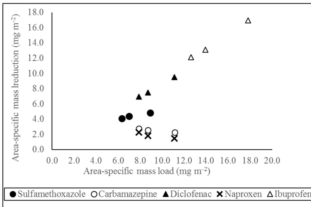
Fig. 2. Area-specific mass reduction as a function of mass load during the whole study period of five pharmaceutical substances in the surface flow constructed wetland system EVA.  $n = 3$ .
