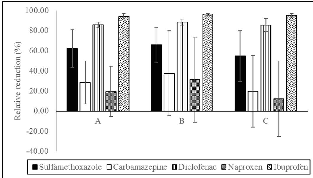
**Fig. 1.** Relative reduction (as % reduction of total loaded mass) of five pharmaceutical substances in the surface-flow constructed wetlands (CWs) consisting of: A) unharvested CWs with mixed vegetation and high mean water depth (0.55 m); B) similar to A) but with low mean water depth (0.40 m); and C) harvested CWs dominated by reed and high mean water depth (0.55 m). Error bars show standard deviation.  $n = 3$ .
